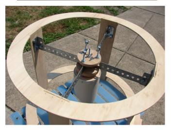
I couldn't avoid building the secondary holder, spider and topside collimation unit any longer. It took a long session on the patio, in the hot summer sun. To my surprise, I had a working topside unit when done. It was constructed of scrap pvc pipe, left over plywood, ½-20 all thread, 4-tee nuts, a short length of steel strap and some hardware store nuts/bolts. I even used some parts from my garage door installation days.
