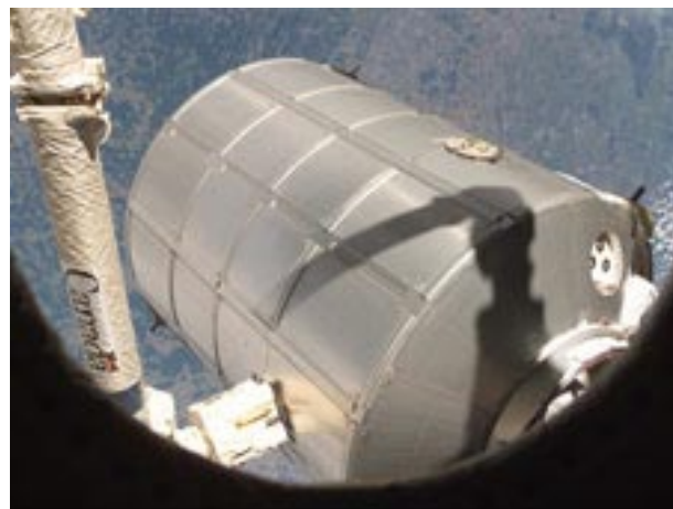
Canadarm2 or the Space Station Remote Manipulator System arm grasps the Italian-built Multipurpose Logistics Module Leonardo to place it back in Discovery's cargo bay. Credit: NASA
