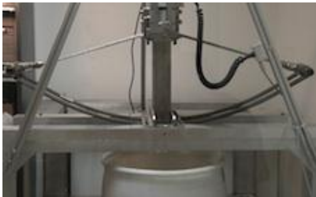
This is a photo of the ballista testbed preparing to fire a prototype harpoon into a bucket of material that simulates a comet. Credit: NASA/Rob Andreoli
