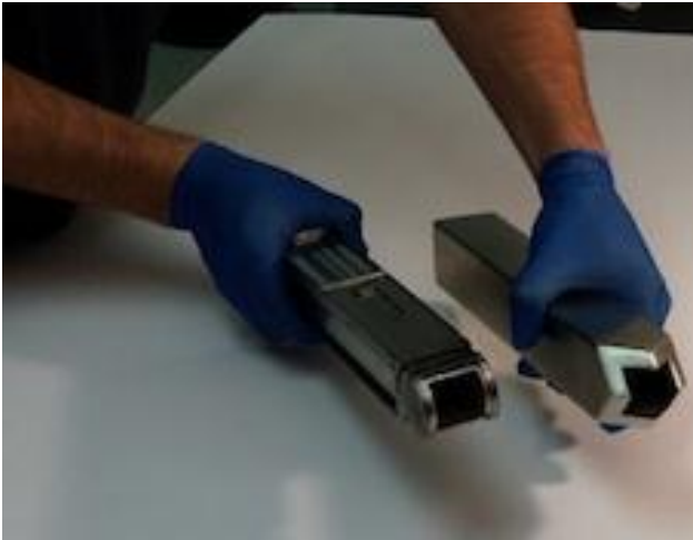
This is a photo of a prototype harpoon tip (right) and sample collection chamber (left). Credit: NASA/Rob Andreoli
